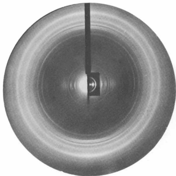
Fig. 1. X-ray diffraction (XRD) photograph of a dried rabbit nerve. The axes of the nerve in all the photographs in this paper are vertical; equatorial reflections are on the horizontal axis, and the meridional reflections are along the vertical axis. The insets in this and the following figures are cut-outs of the bottom films (usually the third) in the film pack. Typical set of d spacings determined from such photographs are listed in Table I.
